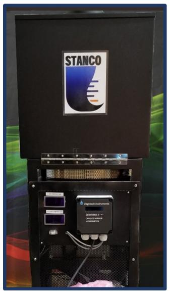
We have extensive experience with closed loop cooling systems in other instrumentation types. We took that knowledge and applied it to carburetor cooling issues of octane engines. To further meet the ASTM requirements, a heavy-duty vaporizer was introduced to ensure that the air stream to the engines is within the required 25-50 grains per pound of dry air. To measure this humidity, a chilled mirror hygrometer is installed to provide constant and accurate readings.
