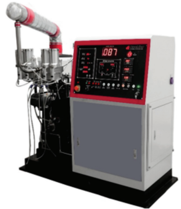
Figure 1: Combination Octane Rating Unit Engine for RON and MON determination of Gasoline
